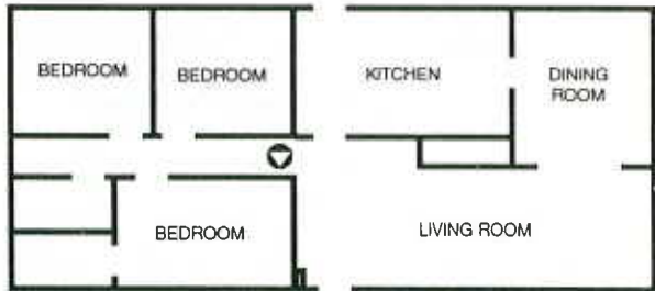
BEST RESIDENTIAL DETECTOR PLACEMENT BETWEEN BEDROOMS AND THE REST OF THE HOUSE
